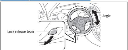
Hold wheel, push lever down, set angle, and return lever. Note: Do not attempt to adjust while the vehicle is in motion.
